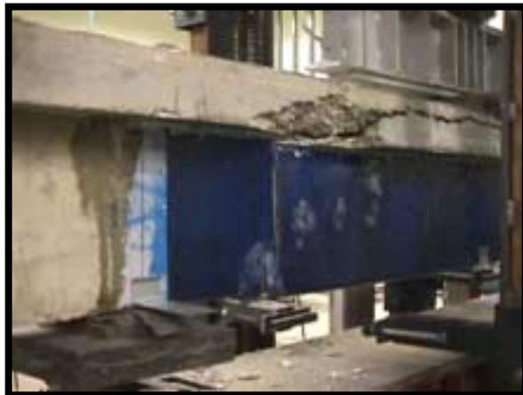
**(c) Beam BT3 (CFRP with end anchors)**
